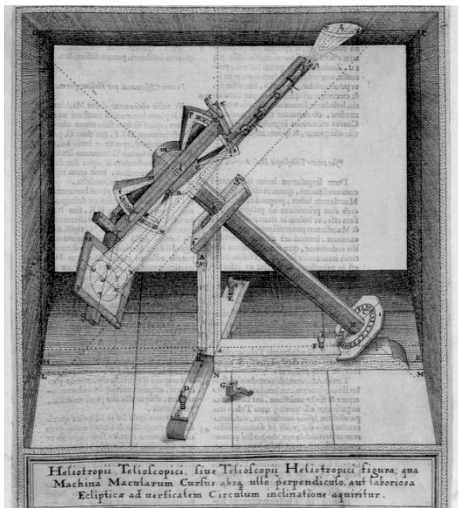
Rosa Ursina: Projection helioscope on an equatorial-type mount
